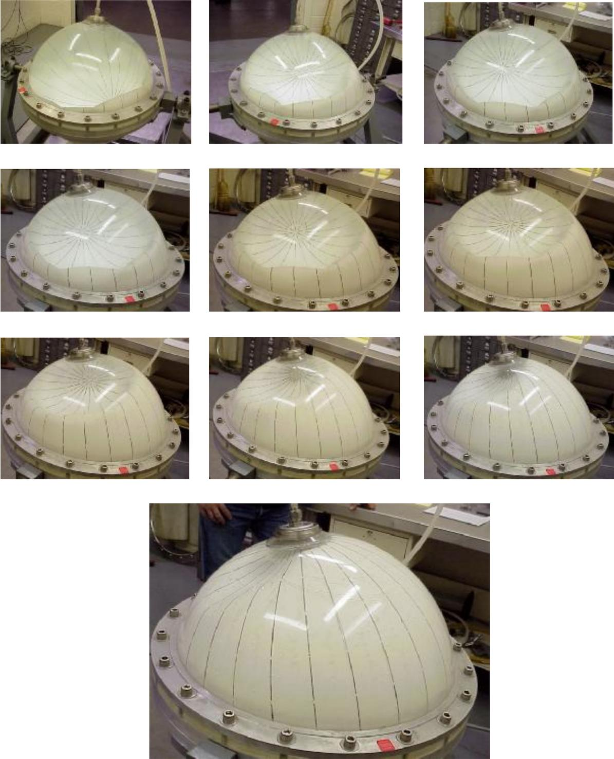
Figure 2: Slosh Test, Stiff Diaphragm
