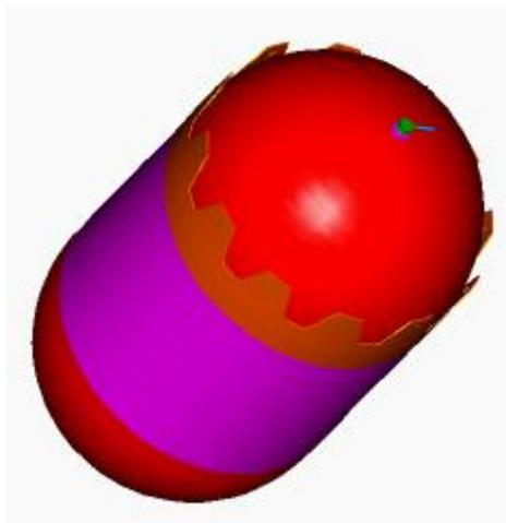
A new PMD, custom designed for the spacecraft mission, was developed for P/N 80425. The passive, all-titanium PMD was designed to accommodate multiple launch environments. The development and qualification of this tank, including the PMD, is presented in detail in Reference 5.
