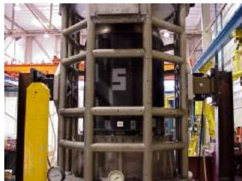
**Figure 11, Dual Shaker Qualification Vibration Test for P/N 80425**
