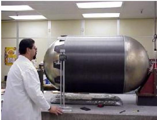
**Figure 12, Liner for P/N 80432**
