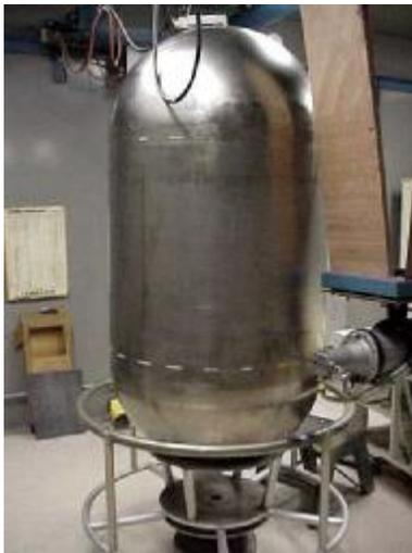
**Figure 8, PSI P/N 80425 liner in X-ray inspection.**
