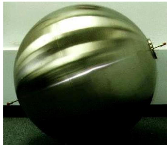
**Figure 1, a Spherical Tank Made From Monolithic STA 6AL-4V Titanium**
