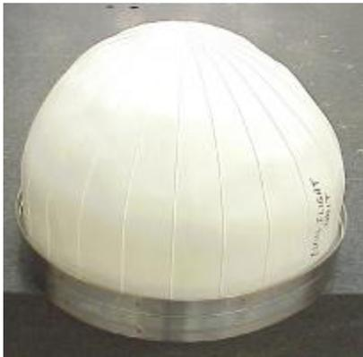
**Figure 17, Diaphragm for P/N 80427**
