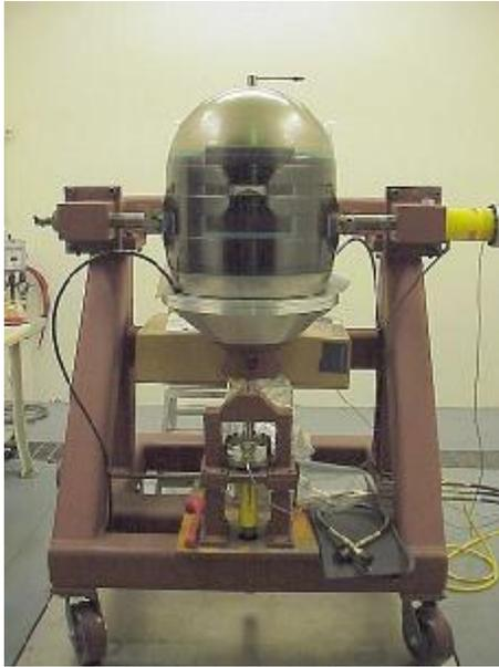
**Figure 20, Static Load Test of P/N 80427**
