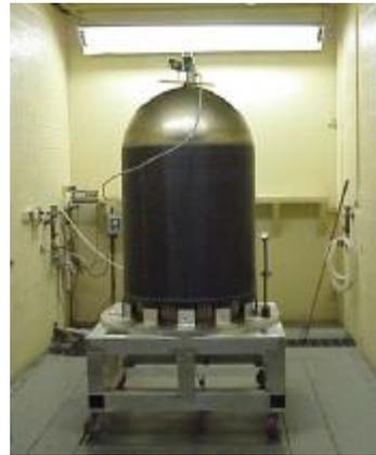
**Figure 10, P/N 80425 with Composite Skirt**
