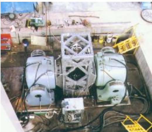
**Figure 7a, Vibration Testing - Lateral**
