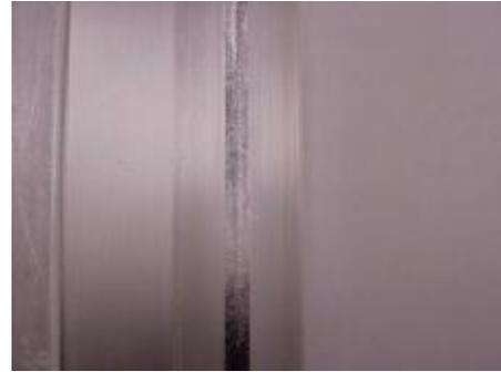
**Figure 4, A Typical Liner Girth Weld**
