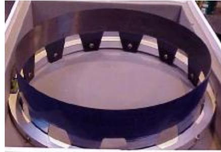
**Figure 9, Composite Skirt for P/N 80425**
