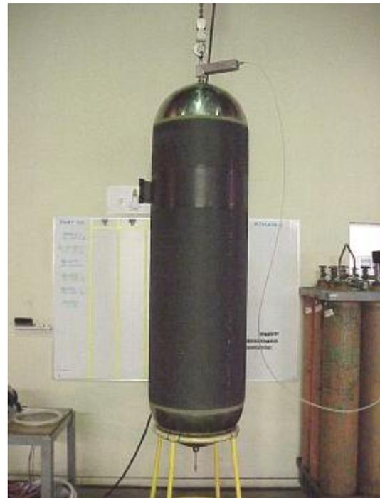
The Hydrazine Tank contains annealed spun domes, which is a deviation from these heritage hybrid propellant tank designs. However, the processes for machining, welding, wrapping, bonding the tabs, and testing all utilized the heritage approach developed for PSI P/Ns 80391, 80395, 80425, 80432, 80434, and 80435.
