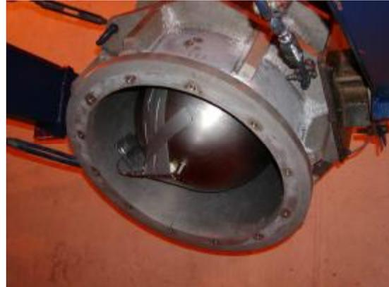
**Burst Pressure Test:** Following NDE and a final visual examination, the Qualification Tank was burst pressure tested to determine the burst margin. The tank burst at 1,292 psig @ 147 °F. The adjusted burst pressure is 1,283 psig at 160 °F, which is 458 psig above the 825 psig requirement. This represents a burst margin of 56%. A picture of the Qualification Tank after burst is shown in Figure 25.
