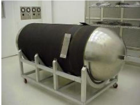
***Figure 2b, Hybrid Propellant Tank, PSI P/N 80432, with Composite Skirt***
