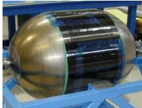
The mounting tabs and anti-rotation tab are bonded to the composite overwrap, followed by a tie-down hoop wrap. The composite is cured. The completed tank is shown in Figure 20.
