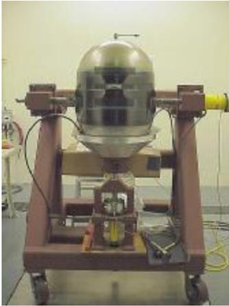
Each tank is subjected to 3 cases of static load testing. Two of the cases test the support tabs and one tests the anti-rotation tab. The test matrix is shown in Table 6. Load Definition is shown below in Figure 23.
