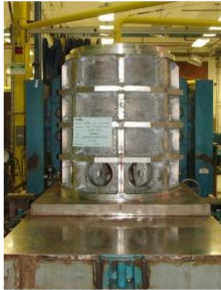
**Pressure Hold Test:** The pressure hold test on the Pathfinder development tank was conducted for approximately 165 hours. The tank was pressurized between 475 (MEOP) psig and 690 psig (proof).
