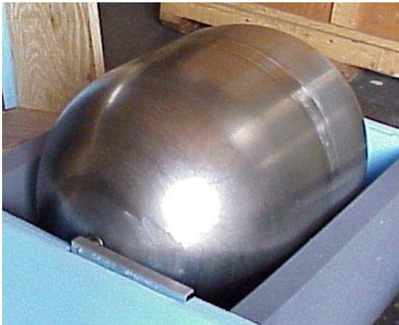
The liner assembly is overwrapped with T-1000 graphite/epoxy composite, over the center cylinder only, as shown in Figure 19.
