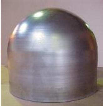
Following spinning operations, the domes were finish machined to achieve final dome contour and thickness, accompanied by anneal and stress relieve cycles to insure dimensional stability. A picture of the finish machined domes is shown in Figure 5.
