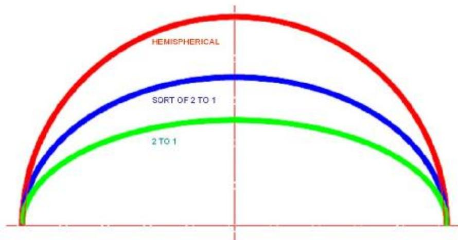
Relatively few all-metal pressure vessels with ellipsoidal heads have been developed. Most of these tanks have  $\sqrt{2}$  to 1 heads. Although all the composite overwrapped pressure vessels developed by ATK has ellipsoidal heads, they were designed to geodesic isotensoid shape<sup>3</sup> to facilitate composite overwrap.
