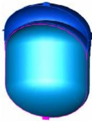
Nested tanks consist of a “typical” tank and an “irregular” shaped tank. The design and manufacture of the “typical” tank presents no new challenges. The design of the “irregular” tank with a concave head is similar to the design challenge of the common bulkhead. Similarly, the PMD design challenges are no different from those of the common bulkhead tank.
