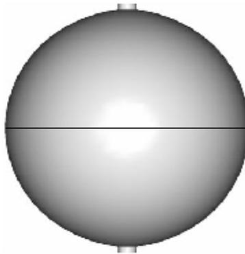
**Figure 1b: Spherical Propellant Tank with Girth Tabs**
