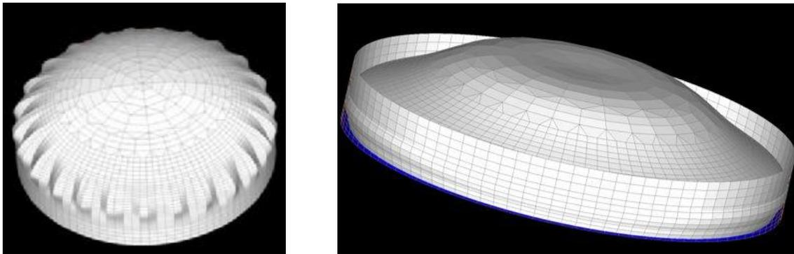
**Figure 6b: Square Root of 2 to 1 Head Buckling Mode**
