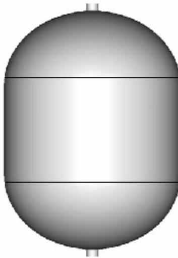
**Figure 3b: Examples of Tanks with Ellipsoidal Heads**
