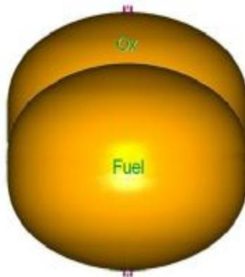
**Figure 10: A Common Bulkhead Tank with Upper Fuel Compartment**
