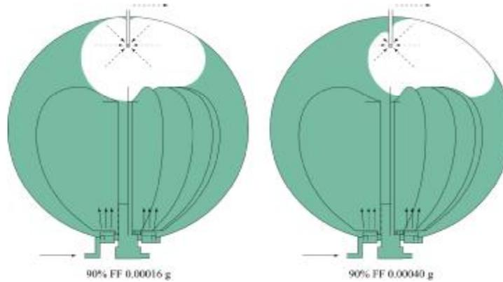
**Propellant Transfer (Gas Acquisition with Lateral Acceleration)**
