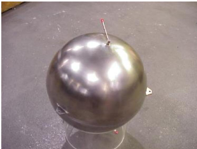
**Figure 8: Hydrazine Tank - Bottom View**
