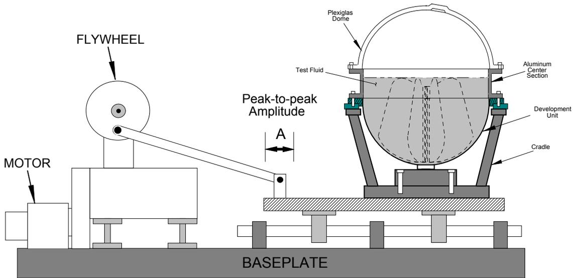
**Slosh test:** A slosh test was performed on the test specimen following the random vibration test. The test setup is shown in Figure 7. An aluminum ring was used to simulate the tank center section, and a 2" thick transparent Plexiglas dome was used to simulate the pressurant hemisphere. The Plexiglas dome allowed visual observation of the PMD and the fluid motion during the slosh test.
