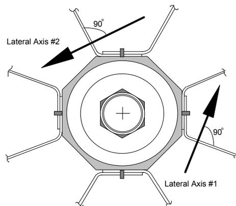
For both Lateral #1 and Lateral #2 axes, and at both 1.7 inch and 3.4 inch input strokes, the resonant frequency remained consistently between 72 and 74 cycles per minute throughout all slosh testing.
