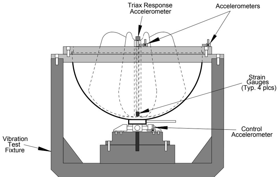
**Figure 5: Stiffness Test Setup**
