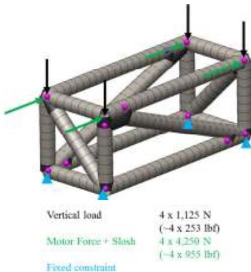
Figure 5. Side Frame loading conditions
