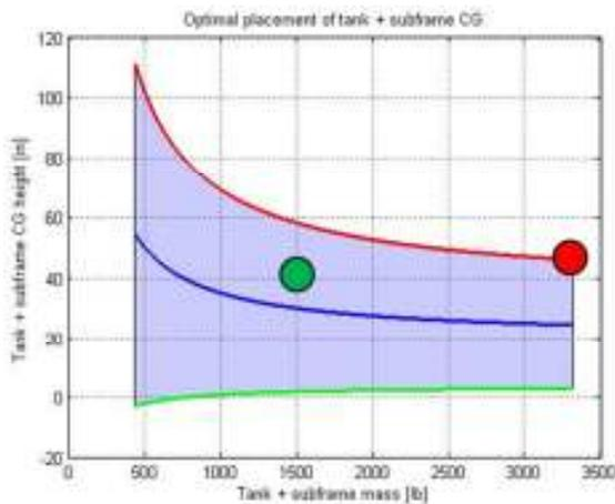
Figure 12. Recommended location of CG. Blue line: Optimal. Green and Red lines: Limit cases
