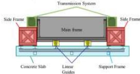
Figure 2. Subassemblies nomenclature. Motion is perpendicular to the page.
