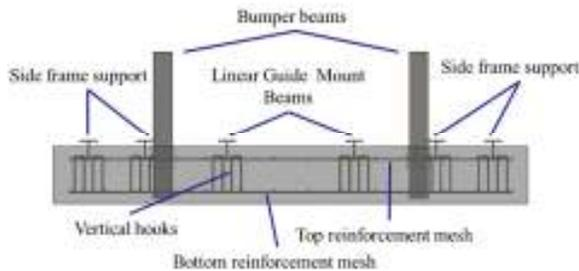
Figure 9. Concrete-embedded support frame section
