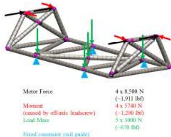
Figure 3. Main Frame loading conditions
