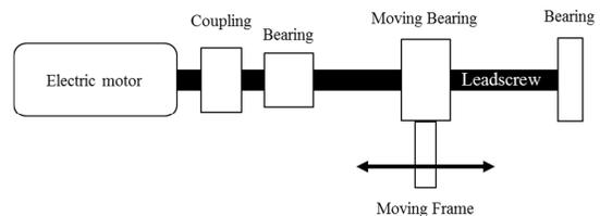
Figure 6. Transmission system diagram
