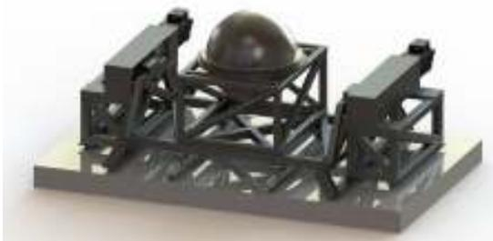
Figure 1. Conceptual 3D model of linear stage, with mock tank and tooling mounted on it.
