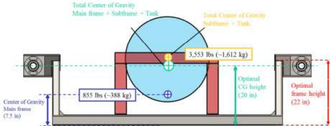
Figure 11. Center of gravity placement
